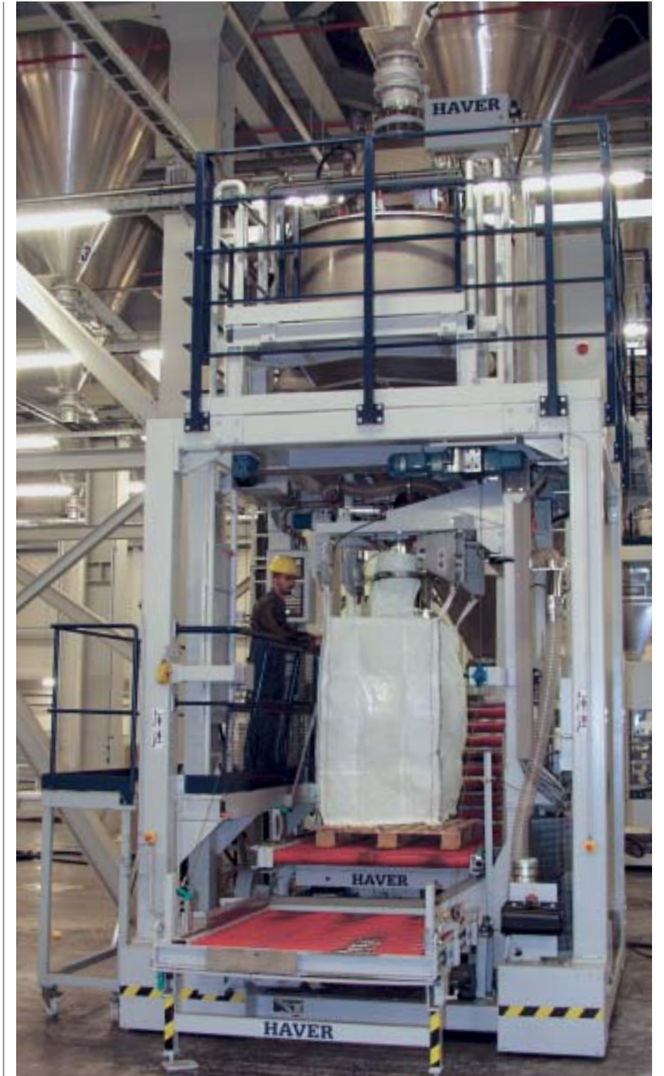
Mobile semi-bulk filling station
