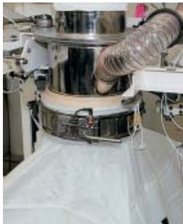
6. Filling spout with an inflatable sleeve (option)
