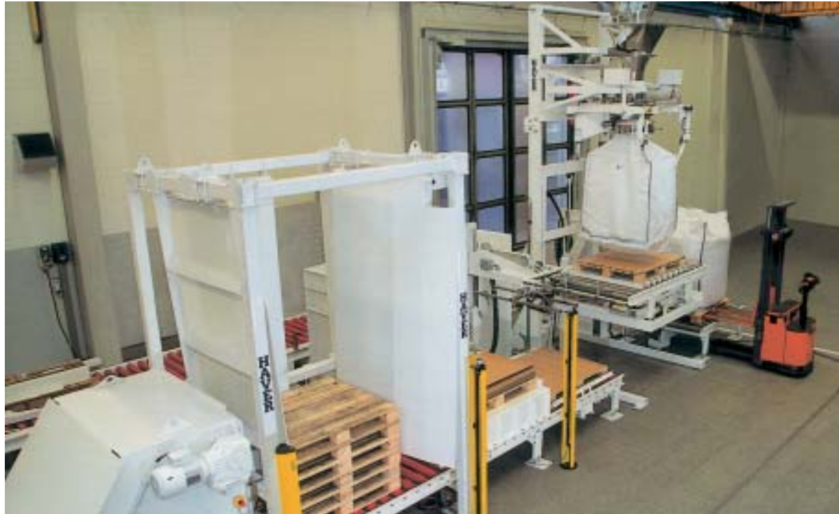
A complete Big-bag filling system equipped with a pallet unitizer, roller system and filling station
