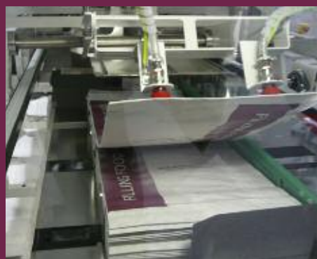
secure: bag separation at the bag bottom for trouble-free operation without bag blockages
