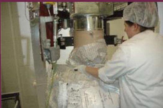
manual closing of the filled big bag – as an option, by our so-called tulip forming
