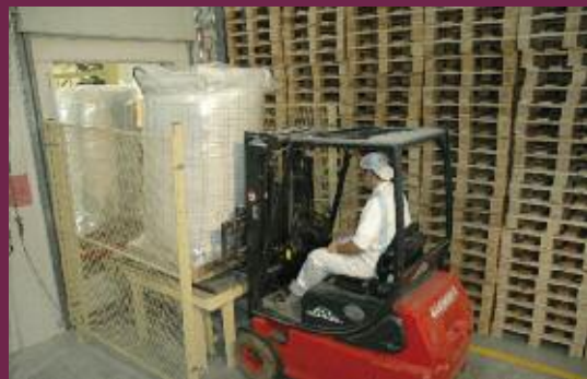
transport of the filled big bag to the full bag storage
