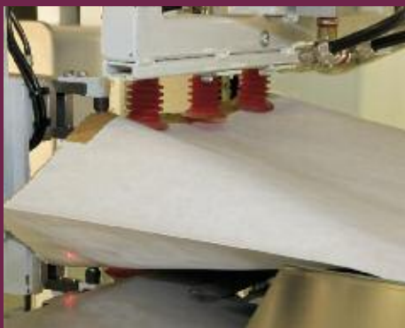
well-proven: bag opening by sucker bars
