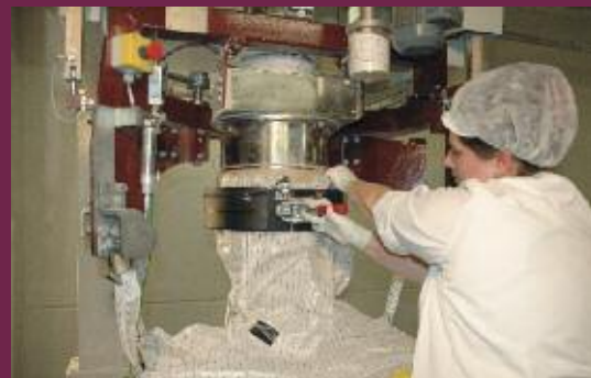
fixing of the filling spout – with inflatable sleeve for dust-tight big bag sealing during filling
