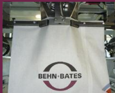
product-specific: bag filling by dust-tight powder or flap type spout
