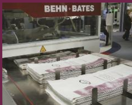
tailor-made: empty bag magazine (maximum capacity: 500 bags)
