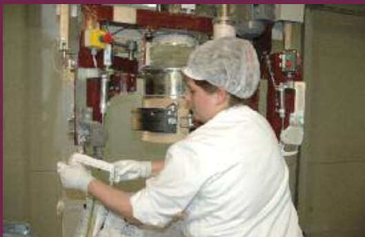
fixing of the big bag loops onto the slewable hooks
